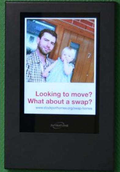
OpenView recommended the installation of a new breed of digital noticeboards that were quick and easy to install as they use GSM technology which eliminates the need for connections to fixed or wireless network infrastructures. Manufactured by Intratone, the units comprise an IP65 rated 15 inch colour screen with options for surface or flush-fit mountings according to the requirements of each location.
